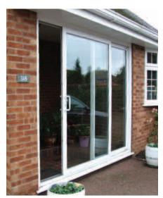
We also offer a specialist "large span" PVC patio door capable of spanning up to 3m per door leaf, this patio is ideal for maximising views with large glass areas and less vertical profile to get in the way. It is also ideal for exposed locations which are susceptible to heavy wind and rain. We are also able to offer this door in a wide range of colours and laminated finishes.
